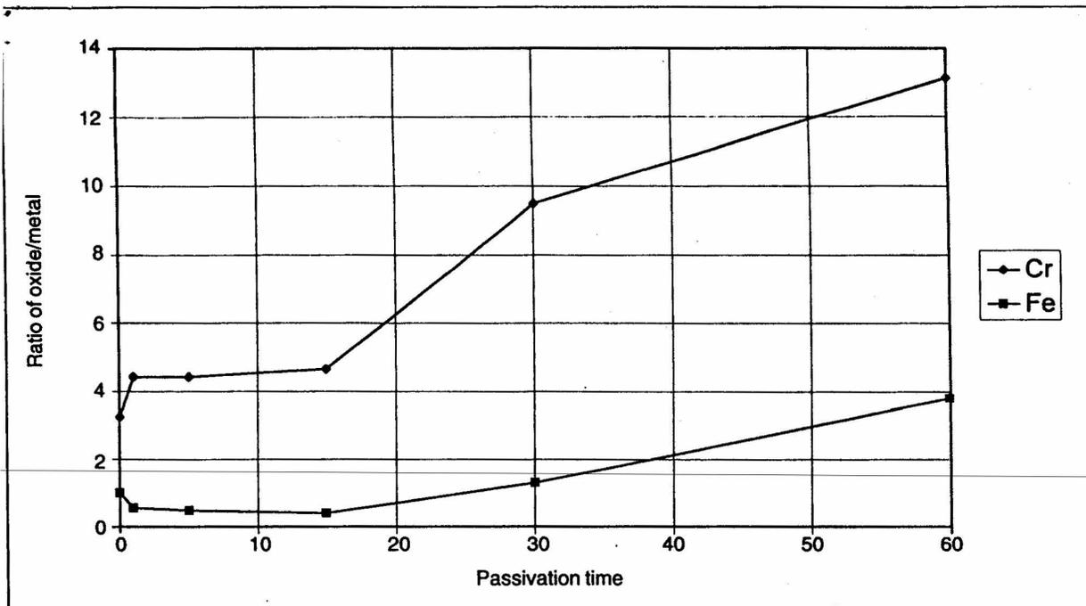
Figure 5: Change in ratio of Cr<sub>2</sub>O<sub>3</sub>:Cr and Fe<sub>2</sub>O<sub>3</sub>:Fe as a function of passivation time
